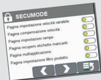
**SecuMode (Security Modeling). Functions and protectable operating parameters individually (pw variables). The standard security can be freely modeled by the client, according to his own organization**
